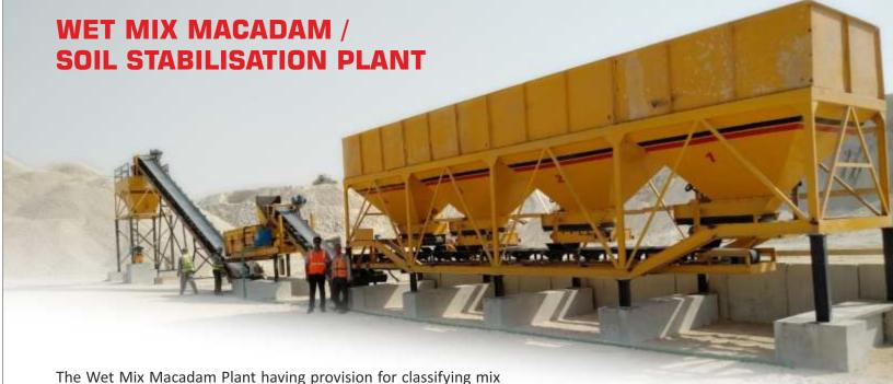
recipe using aggregate of different sizes in the required proportion, addition of specified quantity of water, addition of specified quantity of other ingredients like lime, stone dust or cement and forced / positive mixing of all these ingredients to produce a homogenous mix.
